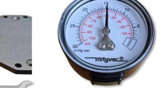
The needle may drop of 1/4" of mercury because of temperature changes
